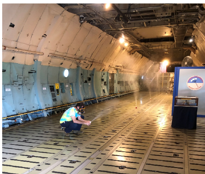
Figure 1. Aerosol testing on a C-5A Super Galaxy airframe located at Dover Air Mobility Command Museum, Dover, DE.
