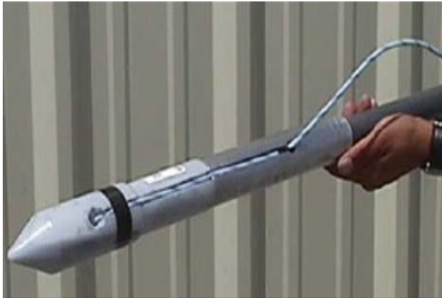
Figure 2e. An explosive ready to be placed. The container is pointed to allow it easily to be pushed into place in a dam, made of plastic to eliminate the possibility of creating a spark, and the top fits easily into a specially made placement rod that allows it to be pushed without the detonating cord getting sheered.
