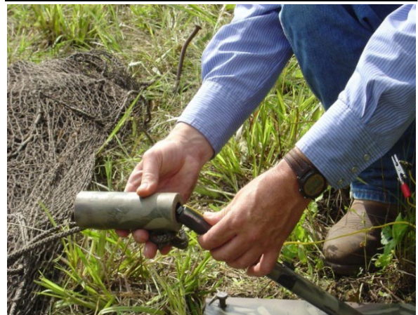
Figure 5b. Cannon net projectile attached to net being placed on launch rod which has a groove for the match leg wires.
