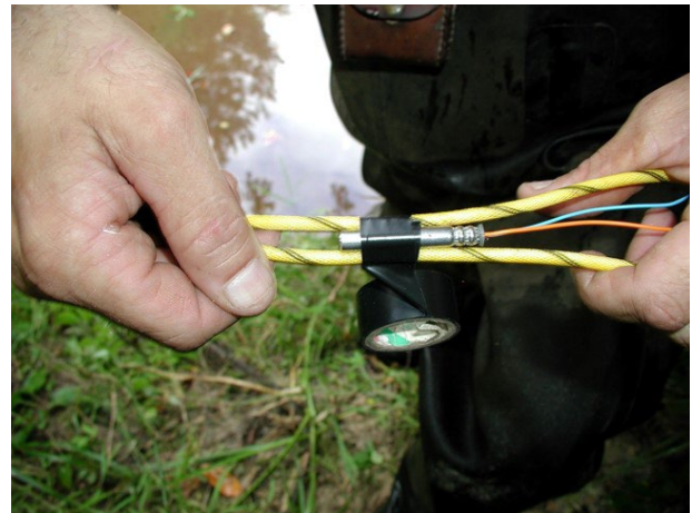
Figure 1b. Attaching a detonator to detonating cord that leads to explosive charges.
