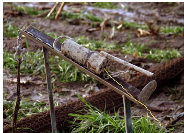
Figure 6b. One of 6 rockets used for project with electric match leg wire coming from an opening where black powder and M-6 propellant are stored.
