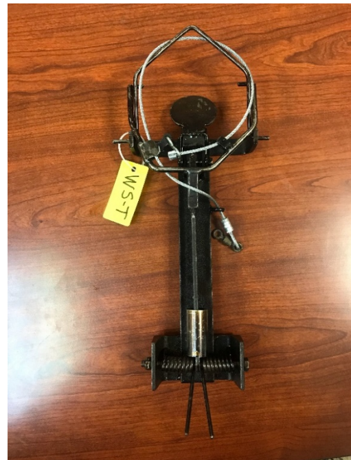
Figure 4. A coyote WS-T foot cable restraint with a WS-T throw-arm, which incorporates a foothold trap pan and pan-tension device.
