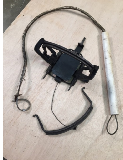
Figure 3. A mechanical foot cable restraint, the “Hold-a-Hog Device,” with a disengaging jaw.
