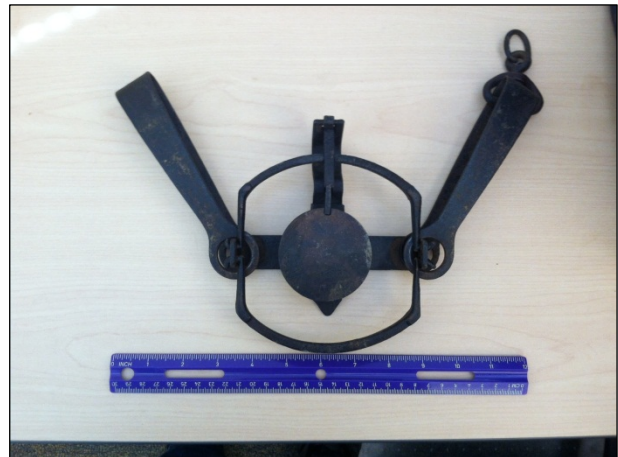
Figure 1. Standard No. 3 trap used by APHIS-WS for trapping coyotes for many years (most have been replaced or laminated to meet BMP standards). This is a double long-spring trap. This is an off-set, metal-jaw trap which is being replaced by padded-jaw- or laminated jaw- traps consistent with best management practices (BMP) standards. The jaw spread is just over 5”.
