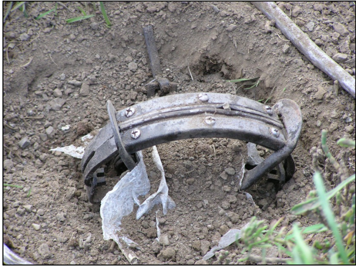
Figure 3. Standard No. 3 padded coil spring trap used by WS mostly for coyotes. This trap is sprung, but in a standard set.
